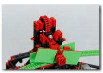
After the ball has been knocked off the magnetic ball holder it rolls into the automatic cross-over which routes all incoming balls alternately to the left and right.
