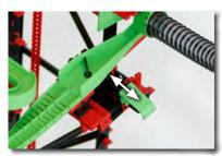
The switch with switch lever are used to determine the direction of the course.
