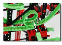
The mechanical switch can be used to adjust the route of the flex-rails.
