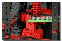
All obstacle courses shown in the assembly instructions include an elevator. This consists of a driven chain fastened to a magnetic ball holder.
