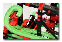
The balls can be stopped at the stopping point and then released.
