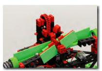
After the ball has been knocked off the magnetic ball holder, it rolls into the automatic cross-over, which routes the balls alternately to the left and right.
