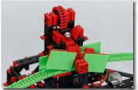
As soon as a ball holder passes by a steel ball in the model's magazine, it is attracted by the magnet and transported to the top. At the top the ball is pushed off and rolls through the obstacle course.
