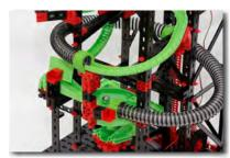
In the rotary funnel the balls from both routes again merge on the subsequent flex-rail.
