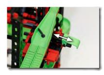
The switch with switch lever are used to determine the direction of the course.
